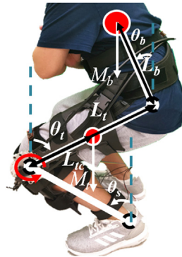
Figure 1.9 Quasi-static model used to derive the assistive knee joint torque during squat motion.
