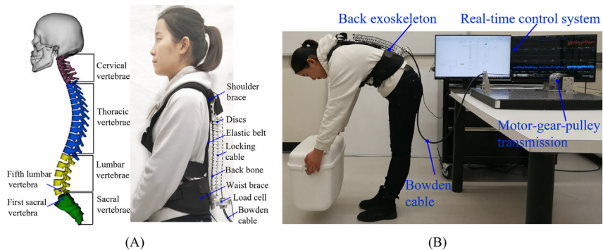
Figure 1.15 (A) The spine-inspired back exoskeleton leverages on a hyperredundant continuum mechanism. Thanks to its compliance, this wearable robot provides assistive force while being conformal to the anatomy of the human back and unobtrusive for natural motion. (B) A healthy subject wearing the back exoskeleton to perform stoop lifting of a 15 kg load. The spine continuum mechanism is powered by a tethered actuation platform via Bowden cable transmission.
